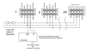
Note: For interconnection of smoke alarms to Fire Panel or Auxiliary devices, use only LIFESAVER Isolation Relay Model RK10A/9.
